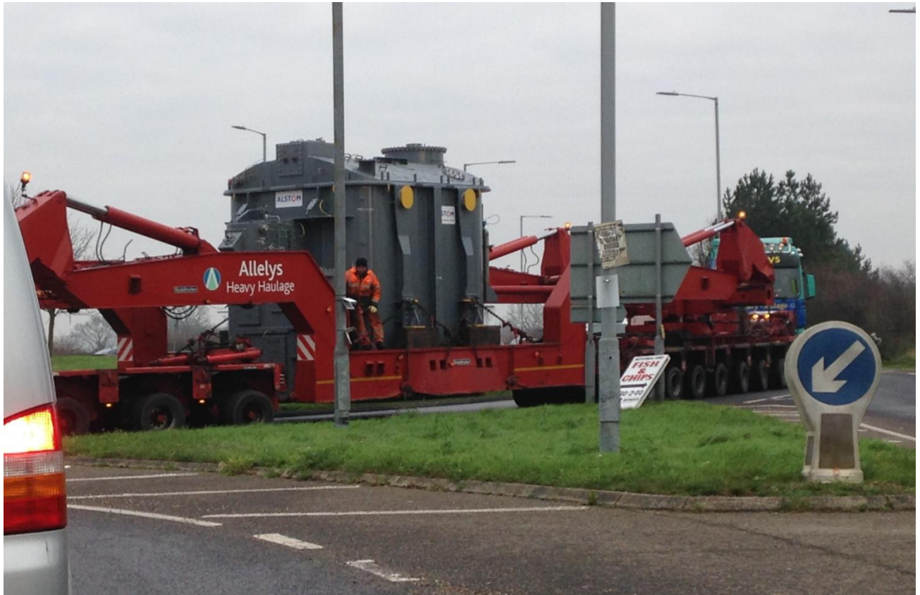
Figure 63. Site 12-13. Heavy haulage transported by prime movers at front and rear on the A12.
