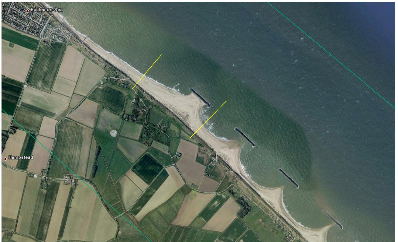
Indicative HDD Alignments for Site 4a (left) and Site 4b (right) in yellow.
