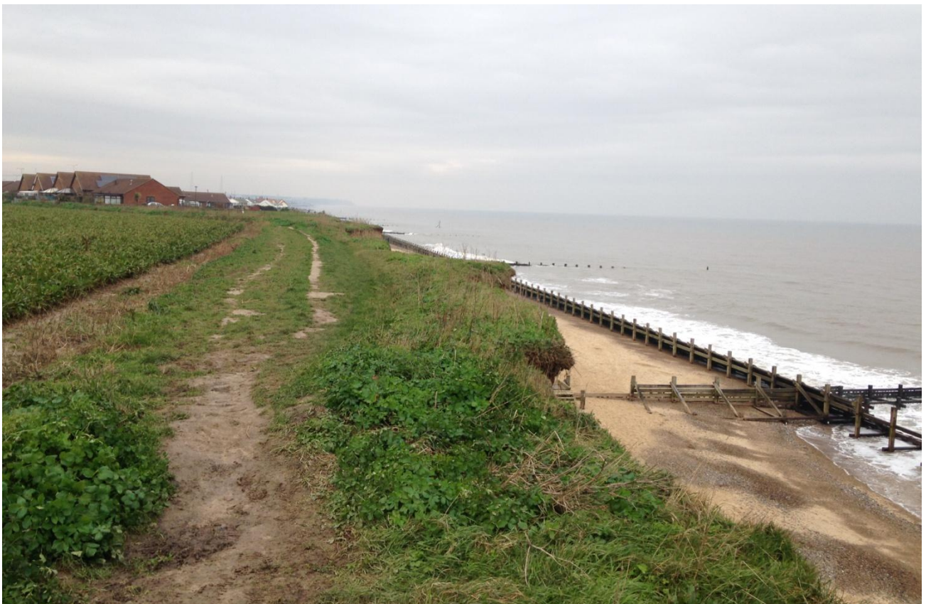
Figure 31. Site 2. View Northward towards Ostend. HDD route is through mid distance with likely entry point to left of photograph, exit point on right between the groins but beyond their seaward end. Note cliff height and coastal erosion.
