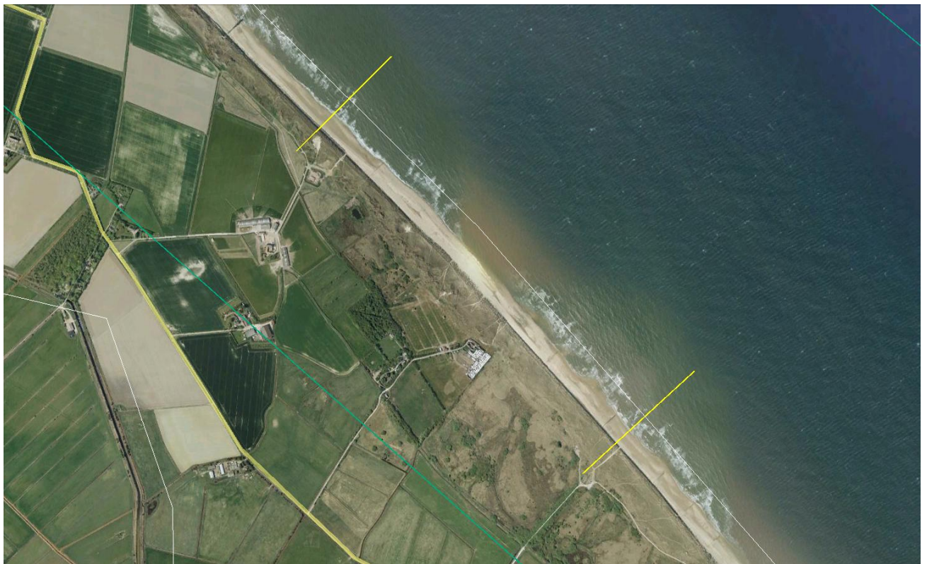
Indicative HDD Alignments near Horsey for Site 6 (left) and Site 7 (right) in yellow.
